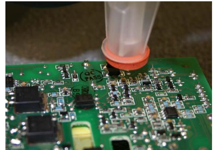
Tip of C3 Test Cell (0.1 in<sup>2</sup> Opening) Being Positioned to PCBA
